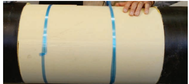
Rigid, pre-formed, polyisocyanurate foam half shell insulation. Note: Foam half shells can easily be cut-to-fit with hand saw.
