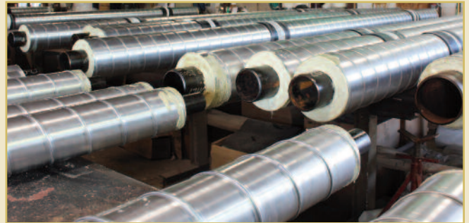
Piping arrives complete with carrier pipe, polyisocyanurate insulation and protective outer jacket – ready to install and resistant to any CUI issues.
