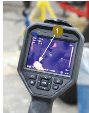
1 Foam being injected – starts to expand from bottom of pipe.
