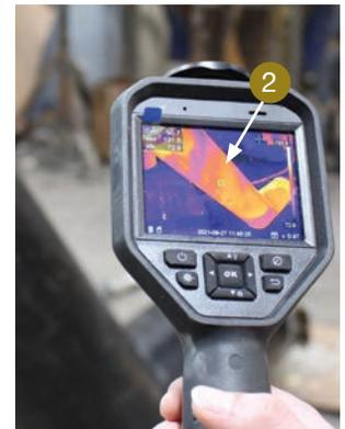
2 Foam expands upward to fill entire air space of piping.
