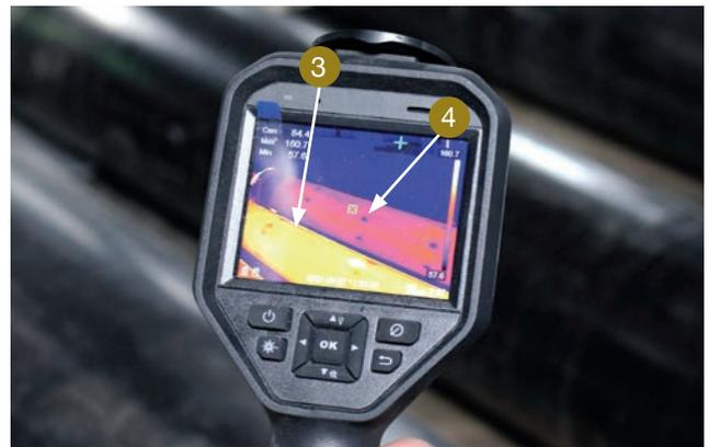
3 Foam expanded and air space totally filled with insulation.
