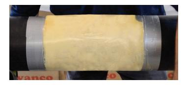
Note: Picture above depicts pipe with open section to show no voids after foam insulation is injected.
