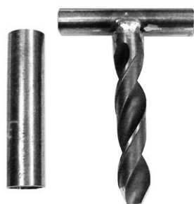
Conical drill \varnothing 28 With distance sleeve
