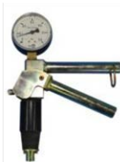
C. Test Instrument for Leakage Tests
