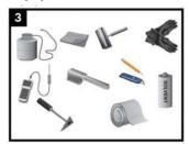
Propane tank, hose, torch & regulator, sandpaper (40-60 grade) or wire brush, knife, roller, rags & solvent cleanser, temperature measuring device, triangular scraper, marking pencil, grater, drill, standard safety equipment, gloves, goggles, hard hat, etc.
