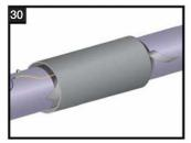
Carefully slide the RhinoJoint over Completely remove the the joint so that the edges are centered over the edge of the adhesive strips.
