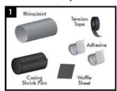
The fully shrinkable Rovanco RhinoJoint is a crosslinked, heat shrinkable casing system for halfshell joint protection of pre-insulated pipes. The RhinoJoint uses an inner shrink film, adhesive strips, rock shield and a tubular casing to seal the joint.
