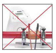
26. During welding, the welding units connecting cable must not exert any force on the fitting.
