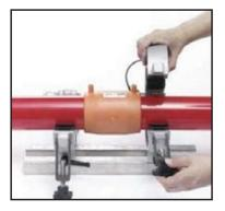
15. After cool down is completed, nipples and universal pipe clamp can be removed.
