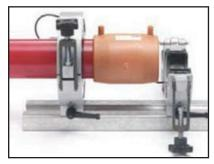
11. Place universal pipe straightening claps as close as possible to fitting.
