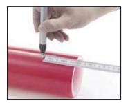
4. Mark scraping area after measuring insert depth of fitting.
