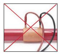
25. Never weld pipe without pre-installed universal mounting clamps.
