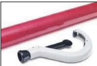
2. Trim pipe to desired length. The cut face must be straight with respect to the pipe axis and must be smooth.
