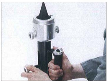
The expander set is fully inserted into the cylinder
