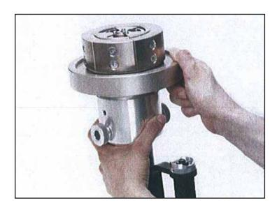
The expander heads 125, 140 or 160 are screwed directly onto the expander set. For this, the expander heads must be fitted so that they are flat and fully screwed in. Avoid any possible tilting when screwing the heads in.
