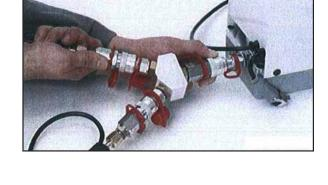
The control cable of one of the two compression cylinders must be connected to the motor (= master cylinder)
