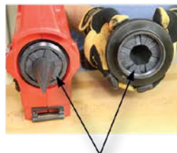
Figure 11: FORCE LOGIC expansion head auto-rotate teeth
