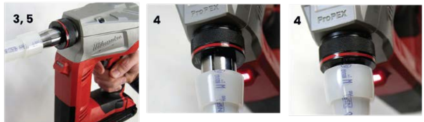
Figure 9: Expansion with Milwaukee M18 ProPEX Expansion Tool
