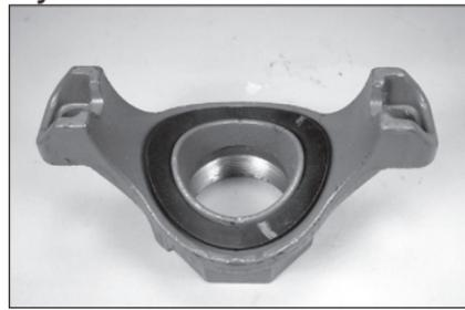
**2a. CHECK GASKET:** Inspect the sealing surface of the gasket to ensure that no debris is present. For Style 920N *Mechanical-T* Outlets, it is not necessary to remove the gasket from the housing. **GASKETS FOR THE STYLE 920 ARE NOT INTERCHANGEABLE WITH GASKETS FOR THE STYLE 920N. THE CORRECT GASKET IS SHIPPED WITH THE APPROPRIATE PRODUCT.**
