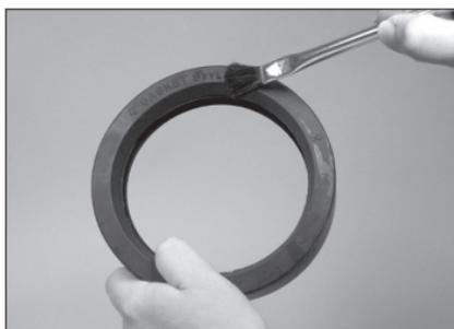
**4. LUBRICATE GASKET:** Check the gasket to ensure that it is suitable for the intended service. The color code identifies the gasket grade. Lubricate the gasket in accordance with the “Lubricant Compatibility for Gaskets” table on page 26. Always consult the pipe manufacturer for lubricant compatibility requirements.
