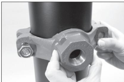
**3b.** Ensure that the locating collar engages the outlet hole properly. Check this engagement by rocking the upper (outlet) housing in the hole.
