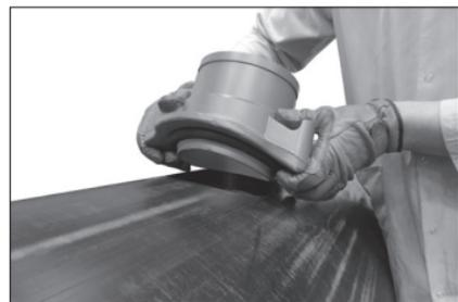
**6. PLACE HOUSING:** Place the housing by inserting the locating collar into the hole in the pipe. Ensure that the o-ring remains in the groove on the housing and does not fall into the hole.
