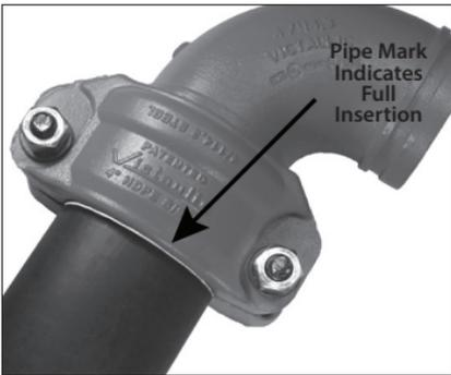
**5a. INSTALL COUPLING:** Wear gloves while handling coupling housings. Retainer teeth are sharp and may cause injury. Assemble the joint by inserting the marked HDPE pipe end into the side of the coupling that is marked “HDPE” and contains the retainer. The HDPE pipe end must be inserted into the coupling until (1) contact with the center leg of the gasket occurs **AND** (2) the mark on the HDPE pipe end indicates full insertion into the coupling, as shown above.
