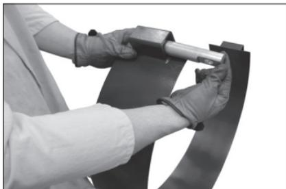
**1. INSERT CROSSBAR:** Insert a crossbar into the retaining bracket on both sides of the strap. The flat side of the crossbar should face away from the open end of the strap, as pointed out in the profile view to the right.
