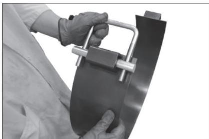
**2. INSERT U-BOLT:** Insert a U-bolt into the crossbar on both sides of the strap. The threaded ends should protrude through the flat sides of the crossbars.
