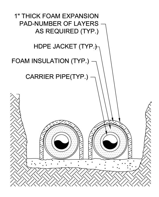
TYPICAL CROSS SECTION W/EXPANSION PADS N.T.S.
