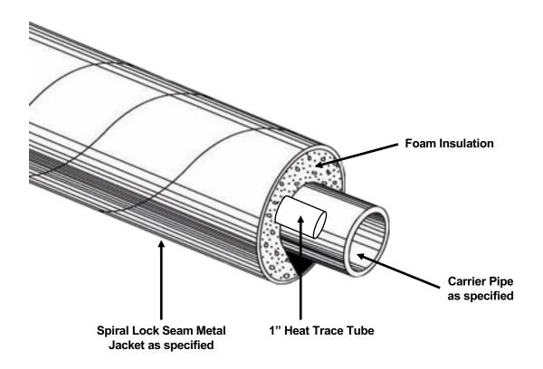
Rovanco's Above Ground Heat Traced Piping is designed for piping above ground suitable for indoor and outdoor applications. Non-Flammable foam insulation and durable metal jacket supplied 20' or 40' random lengths, means an economical, high-quality system.
