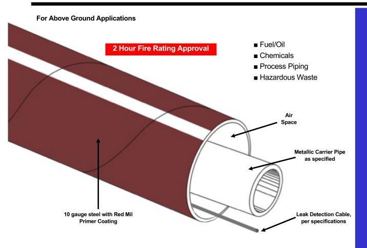
Rovanco's Containment Conduit is designed for piping systems with durable 10 gauge minimum thickness metal conduit. Supplied in 20' or 40' lengths, means an economical, high-quality system.
