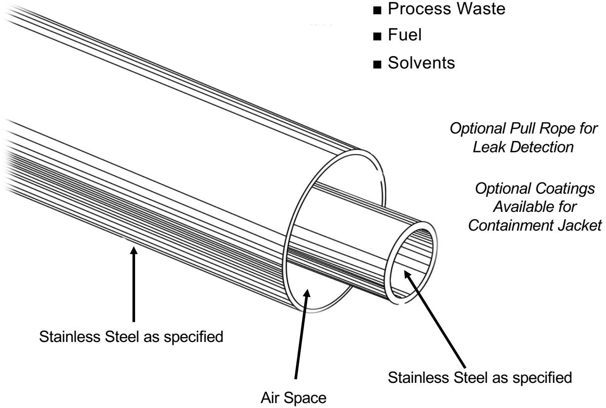
Rovanco's Stainless Steel Containment is designed for piping systems with durable Sch 10 minimum thickness metal containment. Supplied in 20' single random lengths, means an economical, high-quality system.
