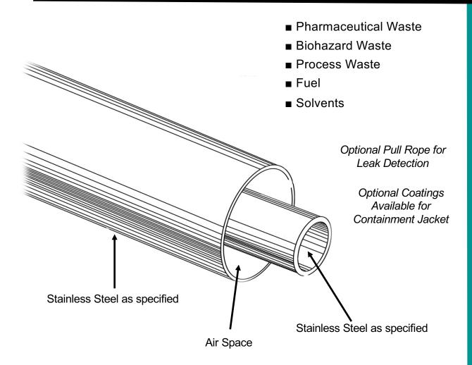
Rovanco's Stainless Steel Containment is designed for piping systems with durable Sch 10 minimum thickness metal containment. Supplied in 20' single random lengths, means an economical, high-quality system.
