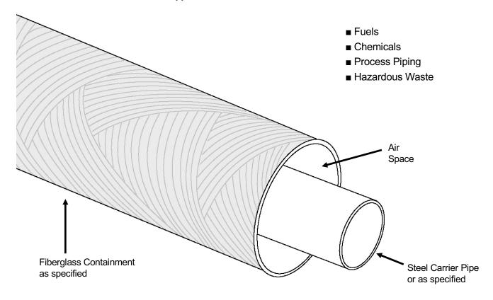
Rovanco's FRP Containment System is designed for applications of high quality with durable FRP casing. All elbows, tees, and end seals are supplied as a standard product for field fabrication.
