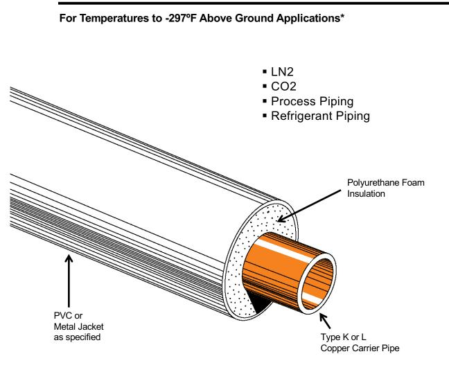
Rovanco's Copper Systems is designed for piping systems above or below ground suitable for inside or outside applications. High quality polyurethane foam insulation combined with a durable watertight jacket supplied in 20' lengths, means an economical, highquality system.
