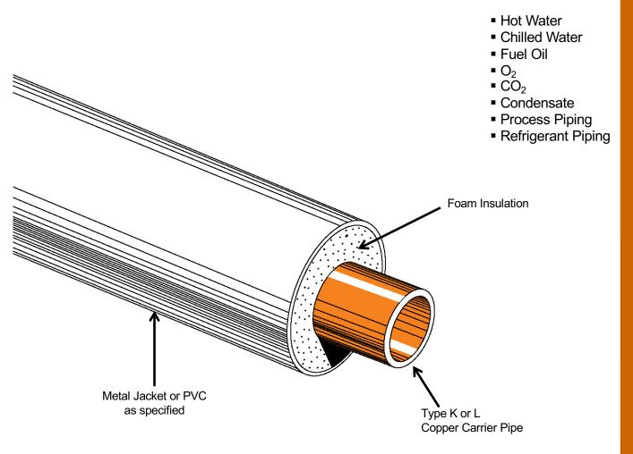
Rovanco's Copper Systems is designed for piping systems above or below ground suitable for inside or outside applications. Carrier pipe insulation is either a polyurethane or polyisocyanurate high quality foam, combined with a durable watertight jacket supplied in 20' or 40' random lengths, means an economical, high-quality system.
