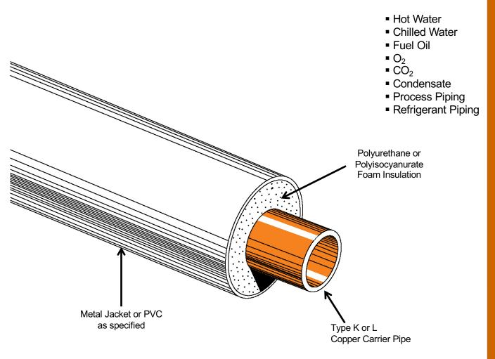
Rovanco's Copper Systems is designed for piping systems above or below ground suitable for inside or outside applications. Carrier pipe insulation is either a polyurethane or polyisocyanurate high quality foam, combined with a durable watertight jacket supplied in 20' or 40' random lengths, means an economical, high-quality system.
