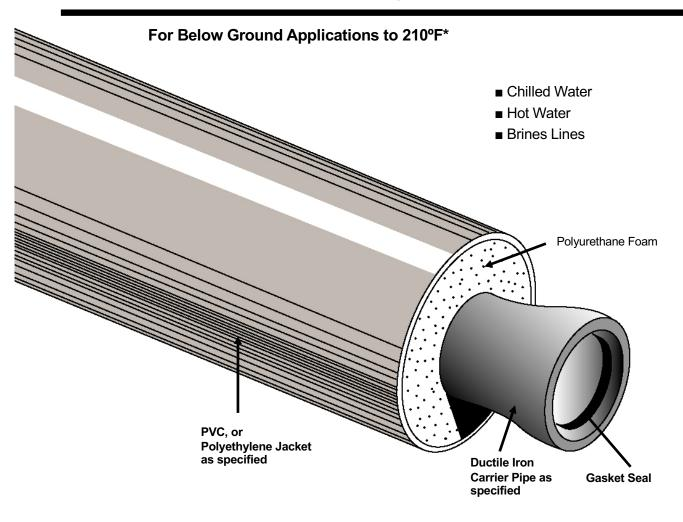
Rovanco's Ductile Iron System is designed for underground applications of chilled water or hot water. Carrier pipe insulation is a high quality polyurethane foam, combined with a durable plastic jacket supplied in 20' random lengths, means an economical, high-quality system.
