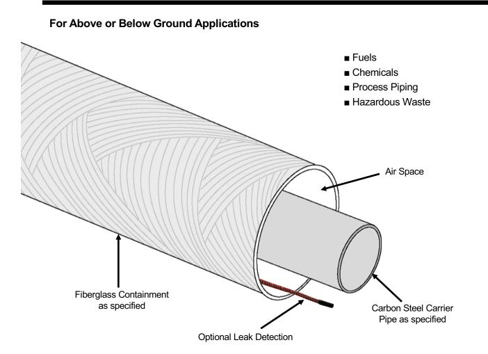
Rovanco's FRP Containment System is designed for applications related to fuel handling with an industry specified Red Thread IIA casing. All elbows, tees, and end seals are supplied as a standard product for field fabrication.
