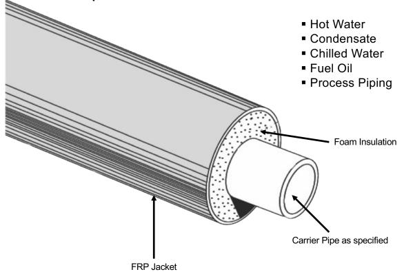
Rovanco's FRP Jacketed System is designed for piping systems above and below ground suitable for indoor\* and outdoor applications. High quality polyurethane foam insulation combined with a durable watertight jacket supplied in 20' or 40' random lengths, means an economical, high-quality system.
