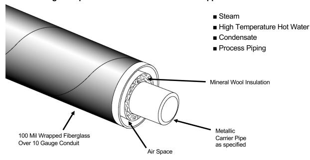
Rovanco's FRP Wrapped High Temp Conduit is designed piping systems suitable for up to 750°F applications. Mineral Wool and a durable 10 gauge minimum thickness steel conduit supplied in 40' lengths, means an economical, high-quality system.
