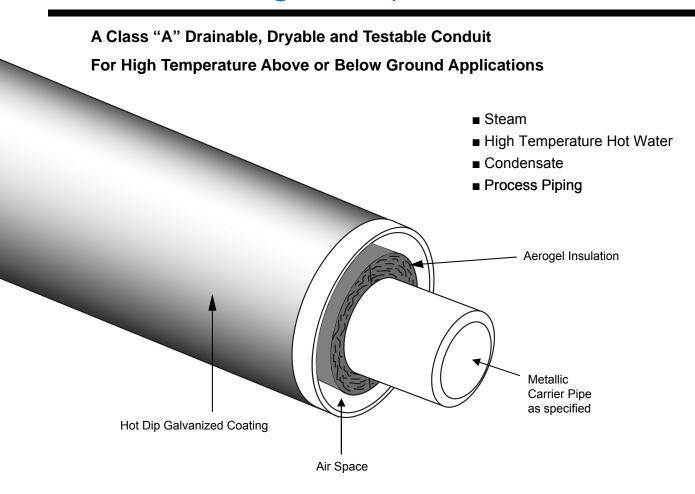
Rovanco's Galva-Coat Temp High Conduit is designed piping systems suitable 750°F for up to applications. Pyrogel insulation, and a durable 10 gauge minimum thickness steel conduit supplied 40' lengths, means an economical. high-quality system.
