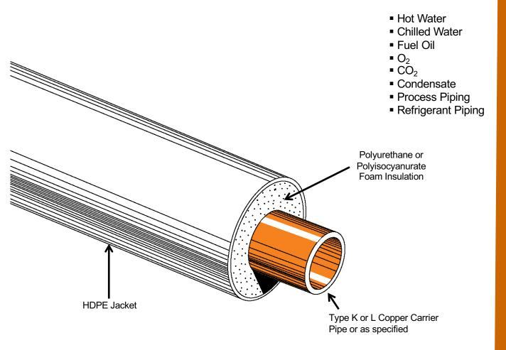
Rovanco's High Density Polyethylene (HDPE) Jacketed System is designed for piping systems below ground suitable for inside and outside applications. High quality foam insulation combined with a durable watertight jacket supplied in 20' or 40' random lengths, means an economical, high-quality system.
