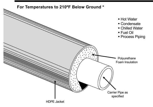
Rovanco's High Density Polyethylene (HDPE) Jacketed System is designed for piping systems below ground suitable for inside and outside applications. Carrier pipe insulation is a high quality polyurethane foam, combined with a durable watertight jacket supplied in 20' or 40' random lengths, means an economical, high-quality system.
