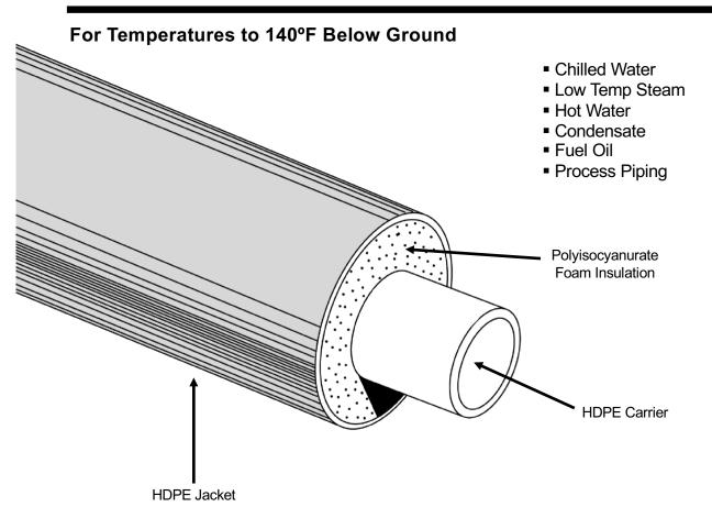
Rovanco's Insul-8 Pre-Insulated Foam HDPE System is designed for piping systems below ground. High quality polyisocyanurate foam insulation combined with a durable watertight jacket supplied in 20' or 40' random lengths, means an economical, high-quality system.
