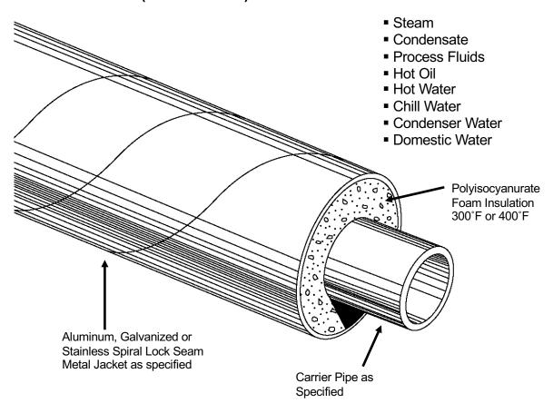
Rovanco's Hi-Temp is designed for above ground, indoor\* & outdoor, piping systems. Insulated with polyisocyanurate foam in combination with a durable metal jacket supplied in 20' or 40' lengths, means an economical, high-quality system.
