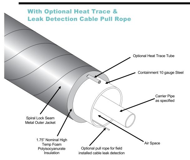
Rovanco's Insul-800 Above Ground Containment with optional Heat Trace and Leak Detection Cable Pull Rope is designed for above ground systems and is suitable for indoor & outdoor applications.
