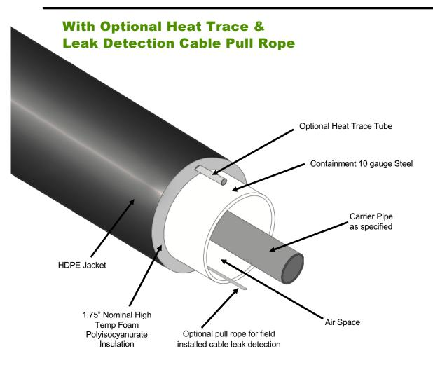
Rovanco's Insul-800 Below Ground Containment with optional Heat Trace and Leak Detection Cable Pull Rope is designed for below ground systems and is suitable for indoor & outdoor applications.
