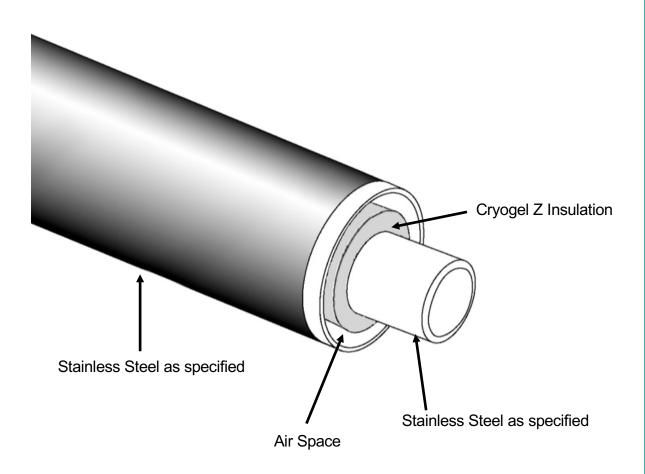
Rovanco's LNG Pre-Insulated Stainless Steel is designed for piping systems with durable Sch 10 minimum thickness metal containment. Supplied in 20' single random lengths, means an economical, high-quality system.
