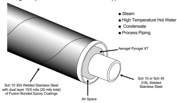
Rovanco's Rhinocoat™ Elite High Temp Stainless Conduit is designed piping systems suitable for up to 750°F applications. Pyrogel XT insulation, and a Sch 10 stainless steel conduit supplied in 20' or 40' lengths, means an economical, high-quality system.
