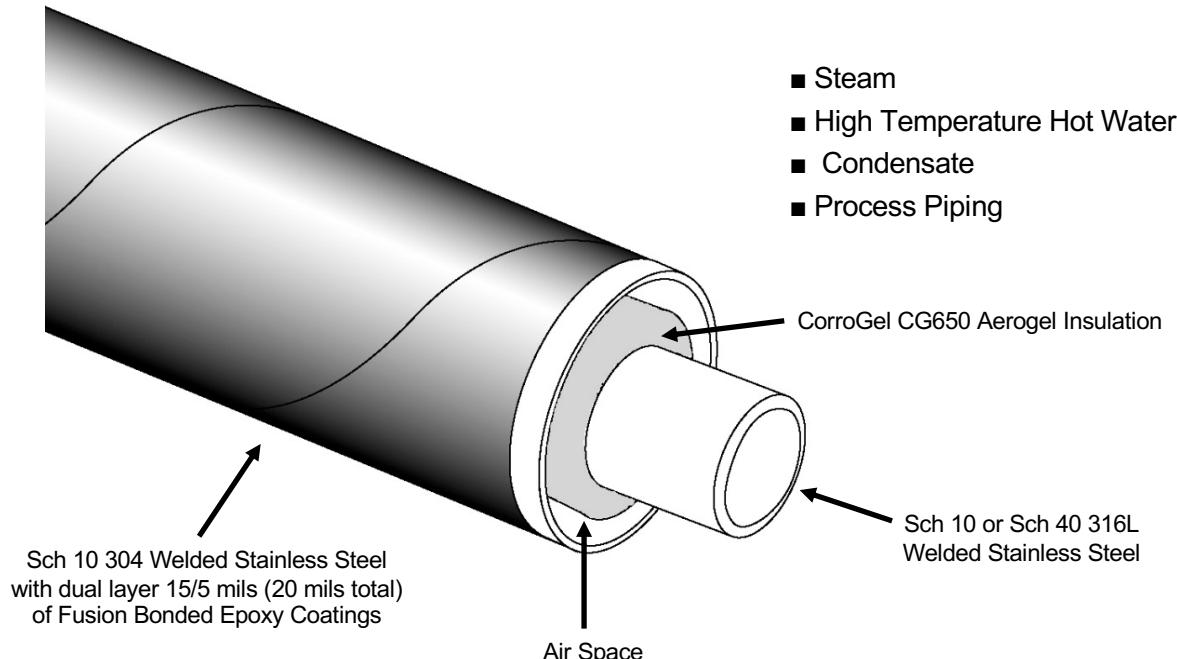
Rovanco's Rhinocoat™ Elite High Temp Stainless Conduit is designed piping systems suitable for up to 750°F applications. Aerogel insulation, and a Schedule 10 stainless steel conduit supplied in 20' or 40' lengths, means an economical, high-quality system.
