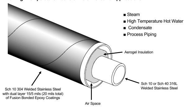
Rovanco's Rhinocoat™ Elite High Temp Stainless Conduit is designed piping systems suitable for up to 750°F applications. Aerogel insulation, and a Schedule 10 stainless steel conduit supplied in 20' or 40' lengths, means an economical, high-quality system.
