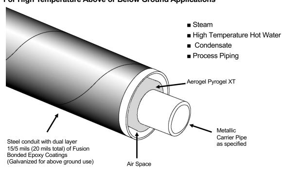
Rovanco's Rhinocoat™ High Temp Conduit Elite is designed piping systems suitable for up to 750°F applications. Pyrogel XT insulation, and a durable 10 gauge minimum thickness steel conduit supplied in 40' lengths, means an economical, high-quality system.
