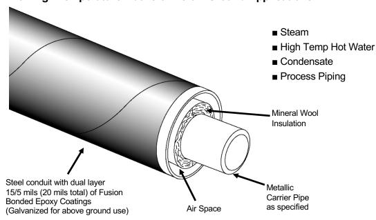
Rovanco's Rhinocoat™ High Temp Conduit is designed piping systems suitable for up to 700°F applications. Mineral Wool or calcium silicate insulation, and a durable 20 mil fusion bonded epoxy coated steel conduit supplied in 40' lengths, means an economical, high-quality system.
