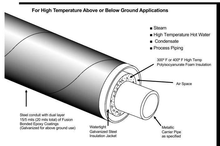
Rovanco's HTF Conduit is designed for piping systems suitable for up to 300°F or 400°F applications. insulation Polyisocyanurate with watertight galvanized jacket covering the foam insulation, and a durable 10 gauge minimum thickness steel conduit supplied in 40' lengths, means an economical, high-quality system.
