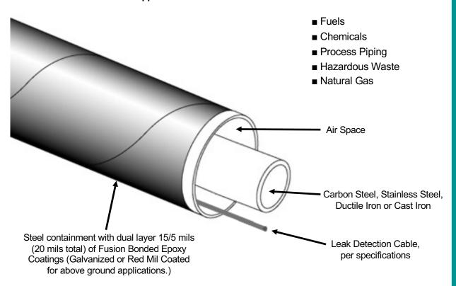
Rovanco's Containment Conduit is designed for piping systems with durable 10 gauge minimum thickness metal conduit. Supplied in 20' or 40' lengths, means an economical, high-quality system.
